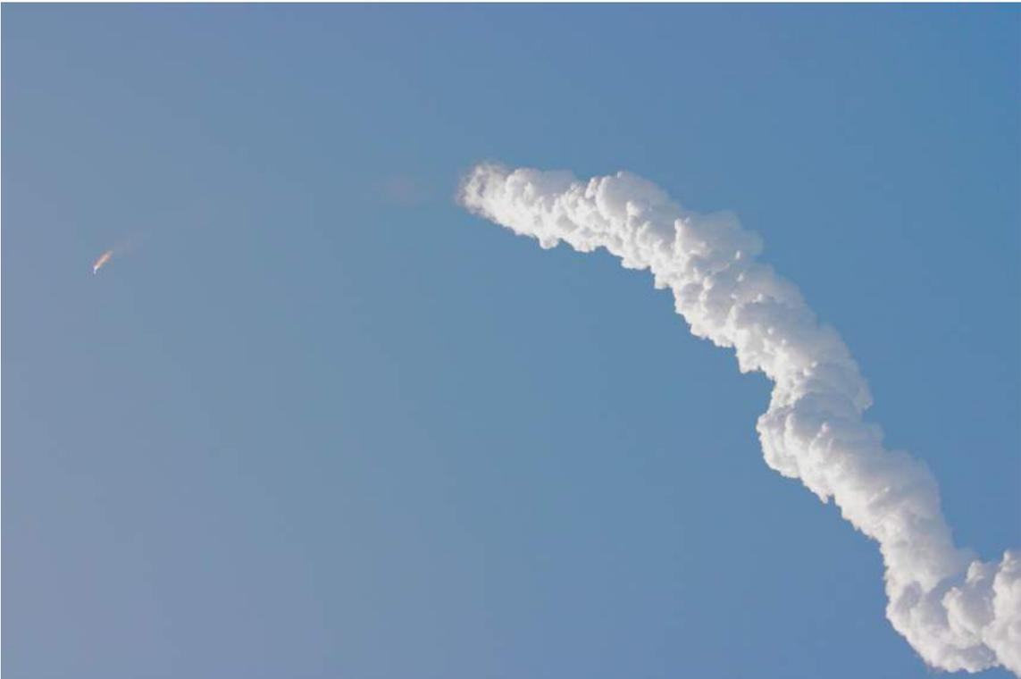
Starship starting to tumble out of control after the failure of stage 2 and a couple of engines
